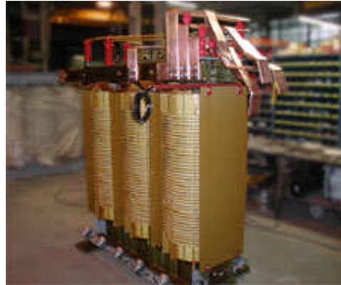
Copper Wire Windings on Transformers
